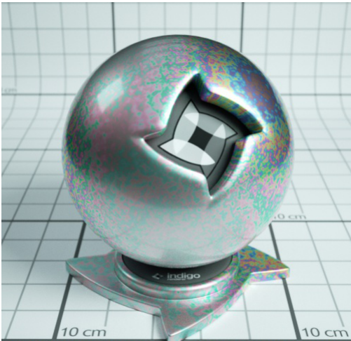
A coating material over a metal metal with interference enabled. Coating thickness is controlled with a shader.
