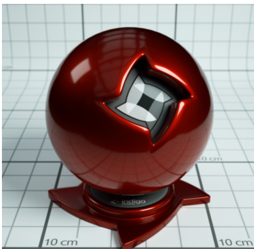
Coating with absorption over a metal material. The red colour comes from the absorption of non-red light as light passes through the coating layer.
